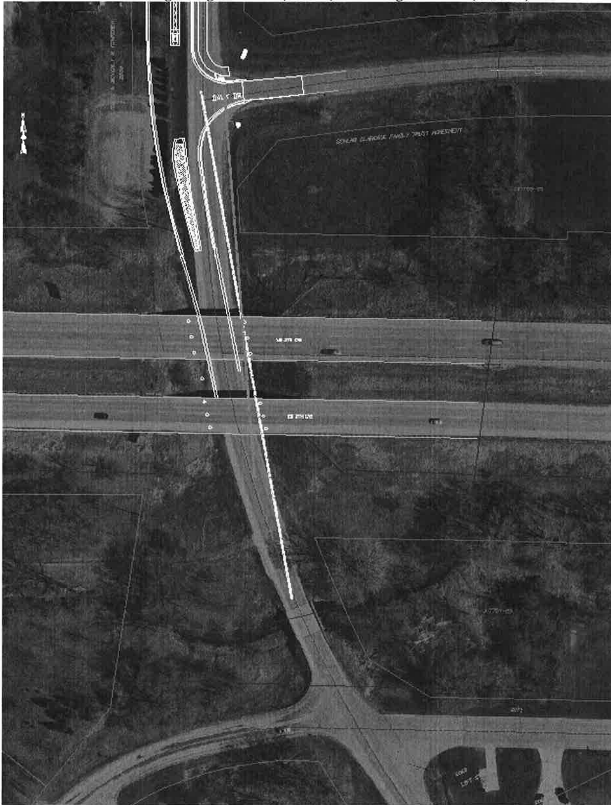
Plan view showing old sight distance (red line) vs. new sight distance (blue line)
